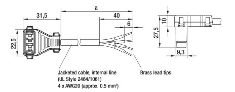
Design: Cable conforms to UL standards, sealed plug. Custom-built connection leads on request.
