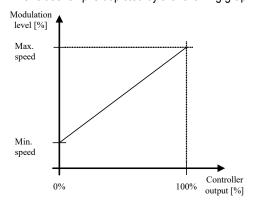
With these parameters, it is possible to set a restriction on the duty cycle (minimum or maximum level).
