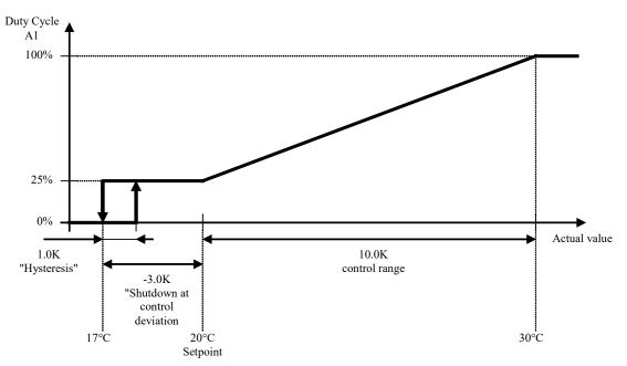
The duty cycle is changed in linear fashion for an actual value in the range [Setpoint .... Setpoint + Control range] = [20°C...30°C] across the range [Min. speed... Max. speed] = [25%...100%].
