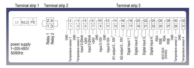
The power supply of the EC Controller is connected to terminal strip 1. Compatible cross-section: 0.08 - 2.5mm² Two relay outputs are connected to terminal strip 2. Compatible cross-section: 0.5 - 1.5mm² The remaining inputs and outputs are attached to terminal strip 3. Compatible cross-section: 0.5 - 1.5mm²
