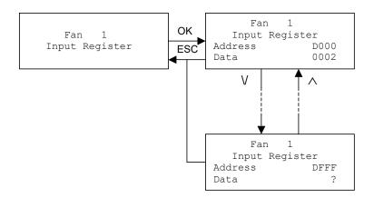
In the "Input Register" menu item, the values of all Input Registers of a fan can be displayed and modified in a range between D000 and DFFF. This is the address range in which all Input Registers of ebm-papst fans typically lie. All values are displayed in hexadecimal format.
