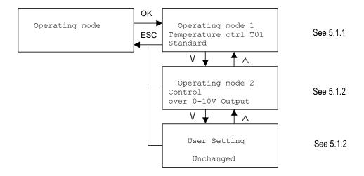
Easy installation of the EC Controller is possible by selecting preprogrammed operating modes (for additional information, refer to 7.)
