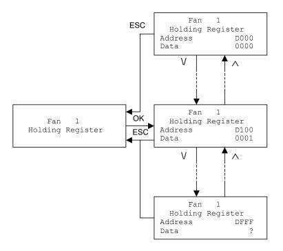
In the "Holding Register" menu item, the values of all Holding Registers of a fan can be displayed and modified in a range between D000 and DFFF. This is the address range in which all Holding Registers of ebm-papst fans typically lie. All values are displayed in hexadecimal format.
