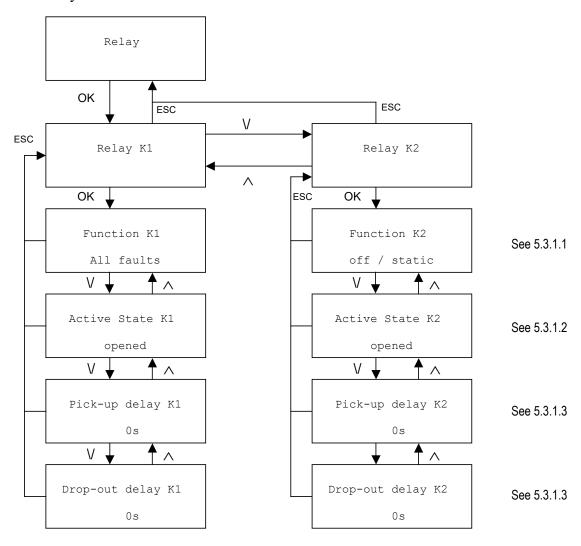
The menu items for relays K1 and K2 are identical in terms of layout. Here, by way of example, is a description of the menu items from relay K1. For the menu items of relay K2, the following applies.
